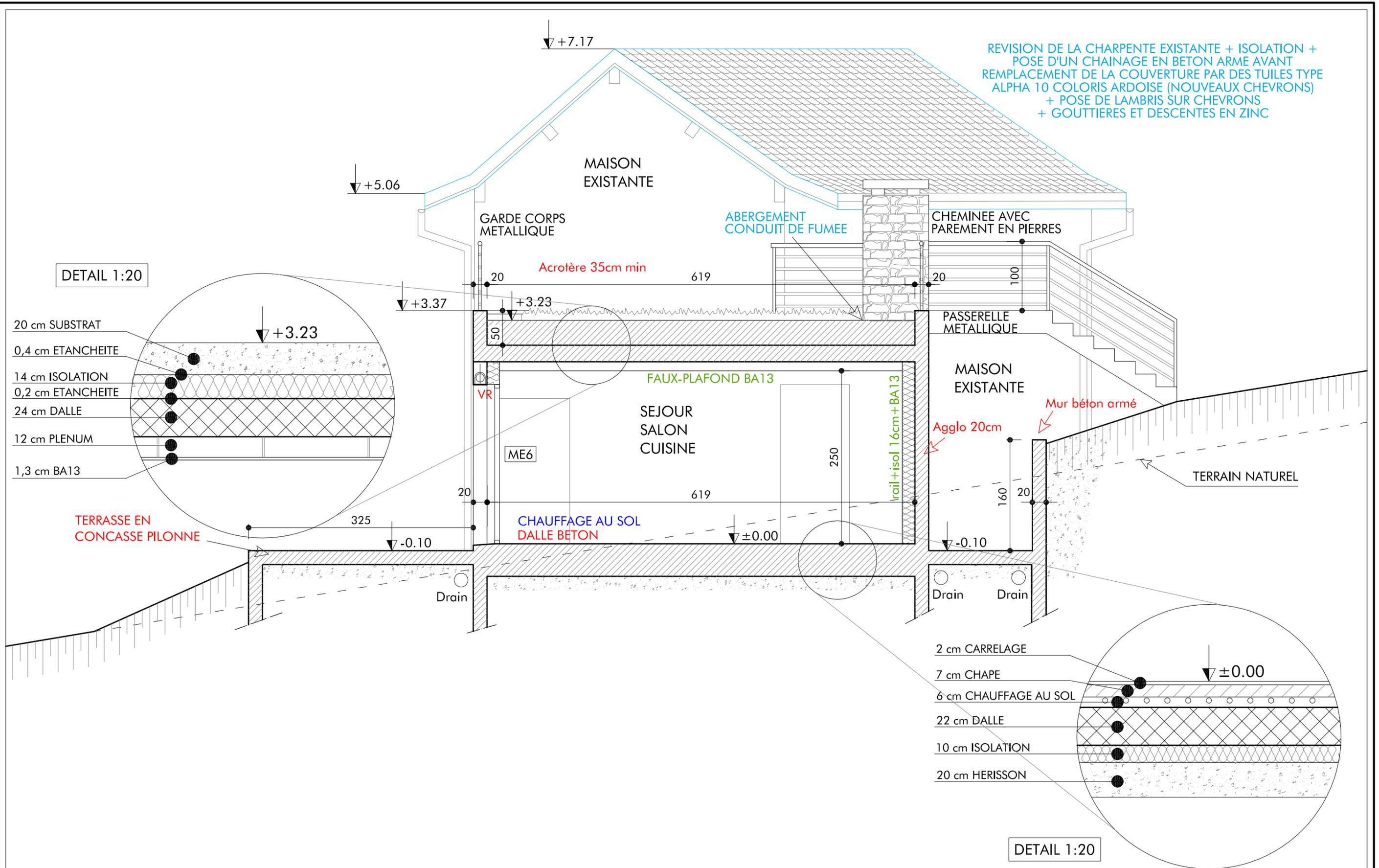
REVISION DE LA CHARPENTE EXISTANTE + ISOLATION + POSE D'UN CHAINAGE EN BETON ARME AVANT REMPLACEMENT DE LA COUVERTURE PAR DES TUILES TYPE ALPHA 10 COLORIS ARDOISE (NOUVEAUX CHEVRONS) + POSE DE LAMBRIS SUR CHEVRONS + GOUTTIERES ET DESCENTES EN ZINC
